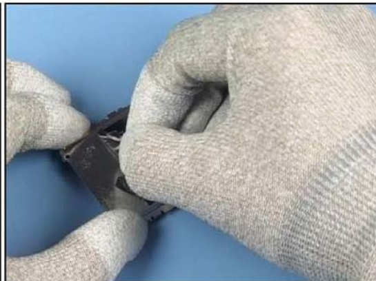
48. Remove any adhesive residues before reassemble.
