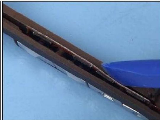
40. Carefully release the glued in CAMERA FLEX ASSEMBLY.
