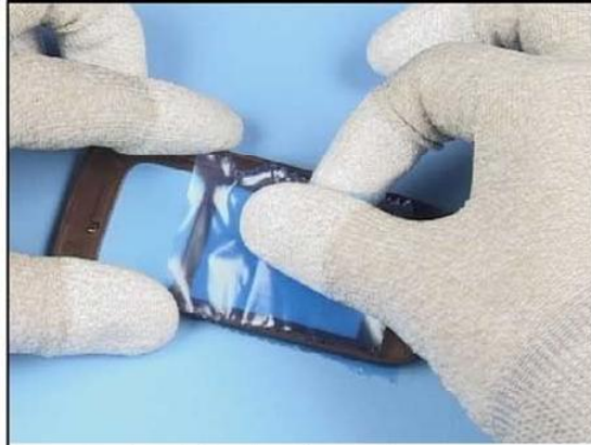
8. Protect the window from inner side.
