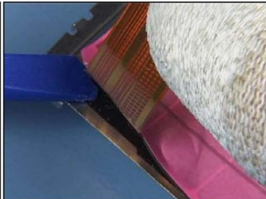
46. Peel up the T9 FLEX ASSEMBLY, beginning from the connector side.
