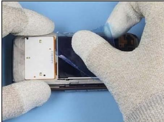
12. Cover the LCD with a protective film.
