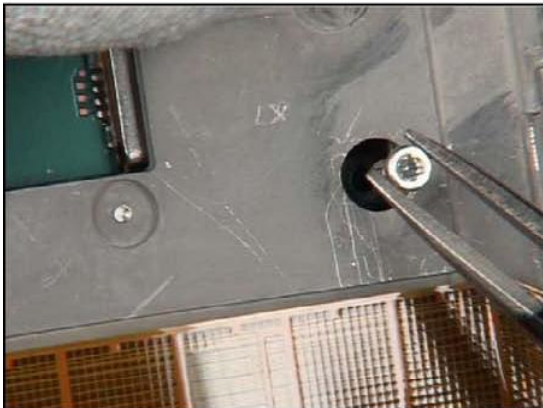
35. Hold the slider into position. Insert the screw.
