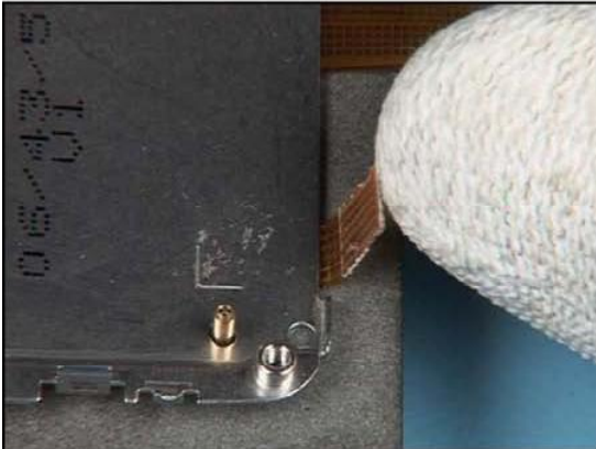
9. Bend over this contact foil and fix it.
