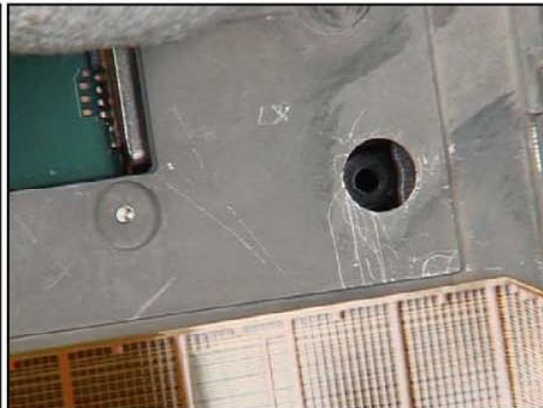
34. Bring the SLIDE MODULE ASSEMBLY into position shown to reach the hidden thread.
