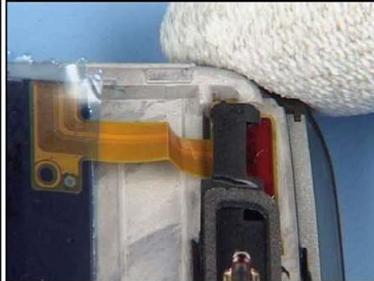
14. Carefully bring it into position shown to gain the maximum flex foil lengths.
