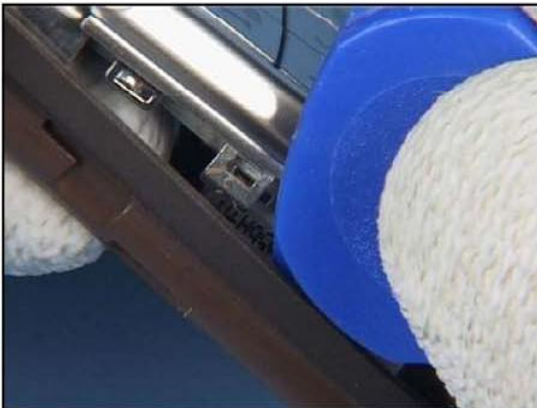
24. Shift open the assembly. Gently pry open these clips of the B-COVER with the SRT-6 in order to reach the clips of the T9 KEYMAT.
