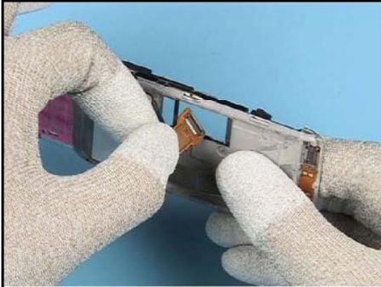
25. Slot the connector through the recess as shown.
