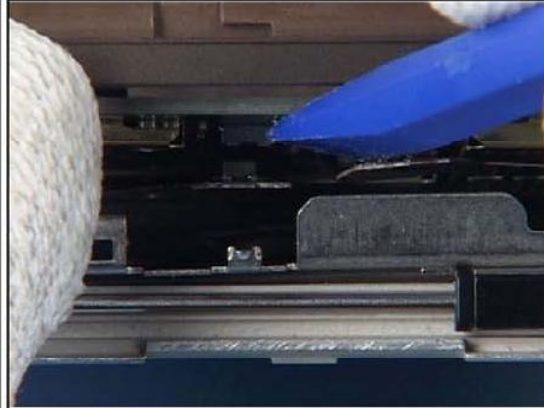
32. Open these 2 connectors with the SS-93 carefully.
