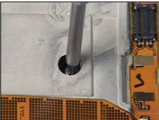
21. Unscrew this screw and remove it before continue.
