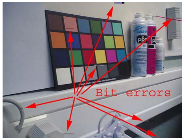
Figure 62 Bit errors caused by JPEG compression
