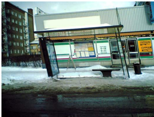
Figure 50 Near objects get skewed when taking images from a moving vehicle
