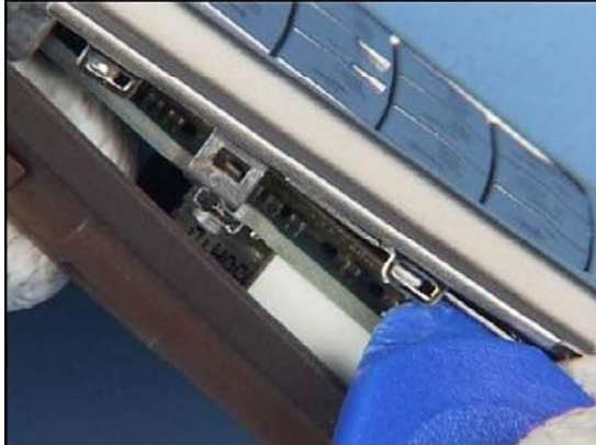
25. Now unlock the metal latches of the KEYMAT...
