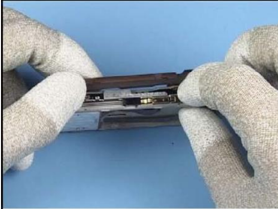
31. Separate the cover slightly. Keep in mind that flex foils are still connected.
