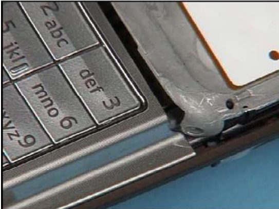
39. Check that the SHEET METAL ASSEMBLY was positioned correctly to ensure the correct functionality of the slider.
