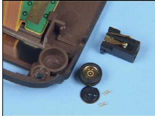
38. Remove the MICROPHONE and the DC JACK. The MICROPHONE will be destroyed surely and must be renewed when reassemble.
